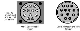
Figure 19 - Baldor motor SSI feedback cable pin configuration
